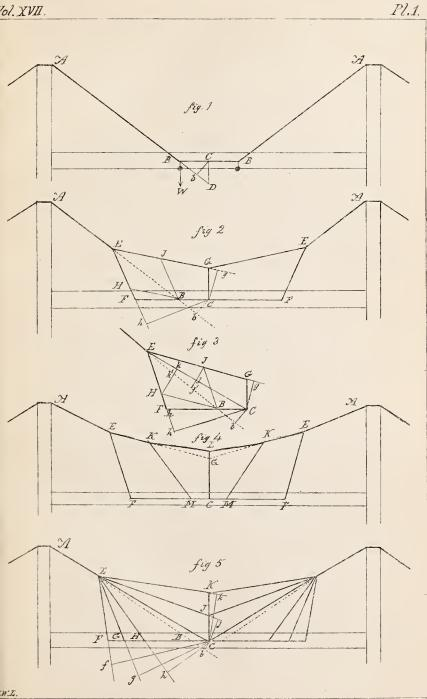
1848.] Quantity of Iron necessary in a Tension Chain Bridge.
